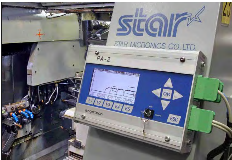
Close-up showing the acoustic fingerprint of an ideal peck cycle for drilling a Hastelloy C-276 sensor component. Boundary boxes where sound presence is mandatory can be seen superimposed on the trace.
