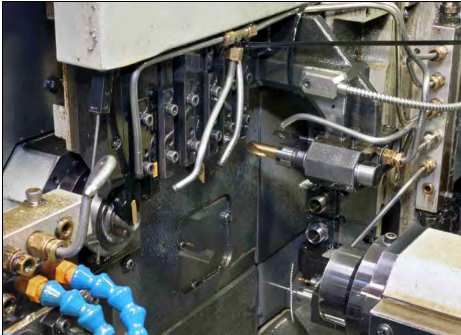
The Argotech acoustic sensor is seen here fitted to the Star lathe platen above the endworking drill. All tools on the platen, including the gang tooling, can be monitored for sound output during machining.
